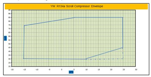
In This Envelop, All Of The Test Condition Under The 11.1  $^{\circ}$ C Superheat, 8.3  $^{\circ}$ C Sub cooling.
