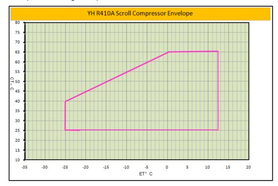
Compressor Running @ 11.1 °C Superheat, 8.3 °C Subcooling
